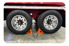
TIRES ✓ 445-50 R 22.5 20PLY tires ✓ Twin 20k rated axles with trailer brakes
