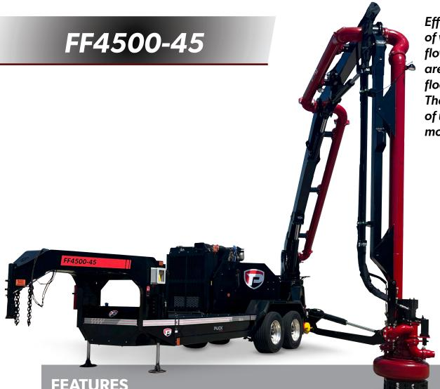
Effective fire suppression begins at the source of water. Utilizing the Puck Force Feed products, flowrates over 4,000 gallons per minute (GPM) are quickly and safely achieved without deploying floating submersible pumps and hydraulic lines. The trailer mounted FF4500-45 creates flow rates of up to 4,500 GPM through a 45' boom and mounted submersible pump.
