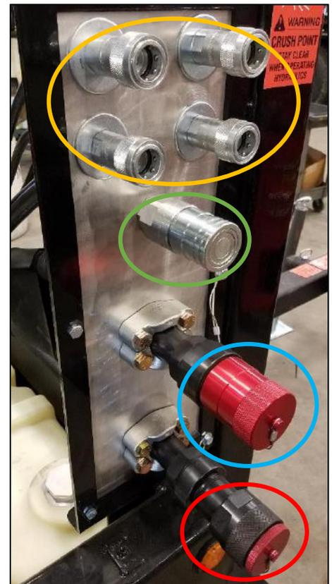
1. When running a new feeder/pump combination together for the first time, always hook up hydraulics on dry land and test first to ensure proper fitment, proper feeder pump rotation, etc. before beginning to set unit in the manure storage. If any issues arise, call your Puck dealer or representative.
