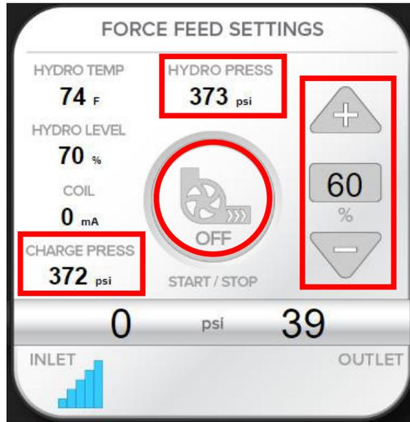
12. Turn the hydrostat on by pushing the pump icon in the middle of the screen.
