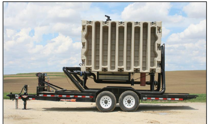
Retracted hinged flotation in position for travel. Transporting, Unloading, and Loading Information
